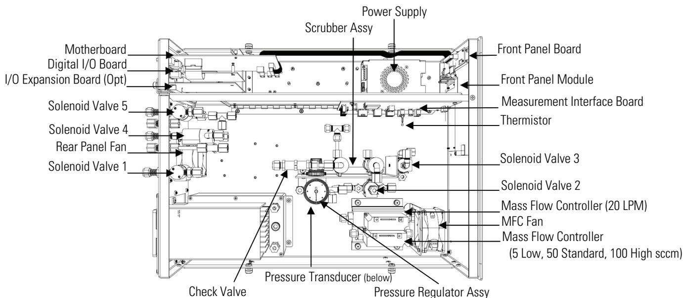
**Figure 7–2.** Model 81*i* Component LayoutCable List
