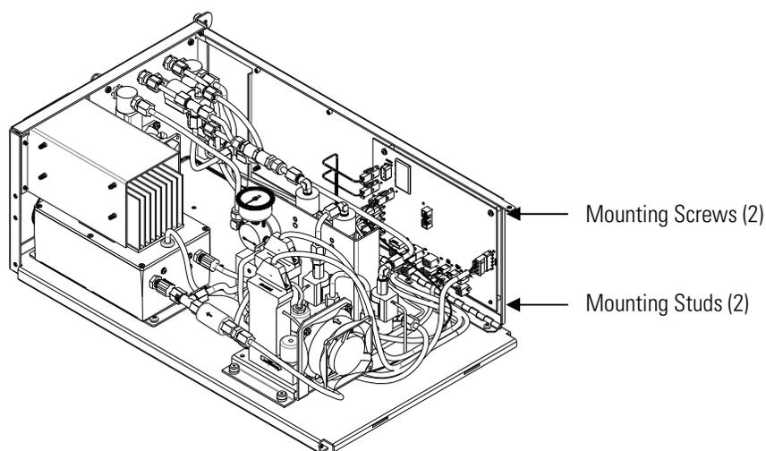
**Figure 7–13.** Replacing the Measurement Interface Board
