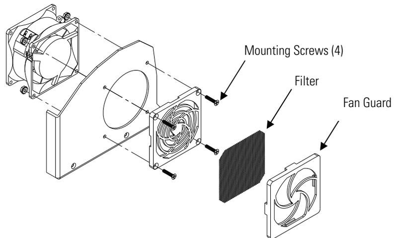
**Figure 5-1.** Inspecting and Cleaning the Fan Filters
