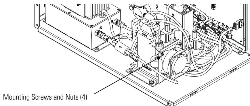
**Figure 7-5.** Replacing the MFC Fan
