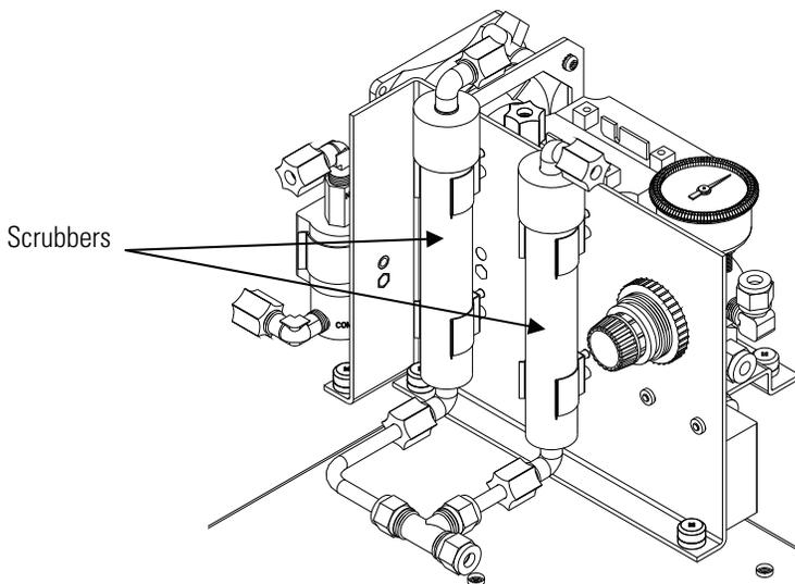
**Figure 7-10.** Replacing the Scrubber
