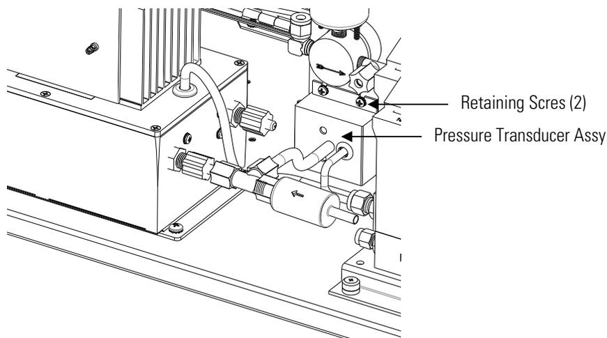
**Figure 7–9.** Replacing the Pressure Transducer Assembly
