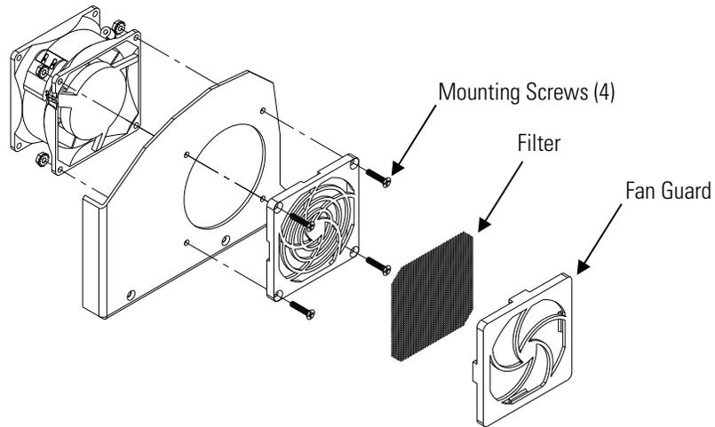
**Figure 7-4.** Replacing the Rear Panel Fan
