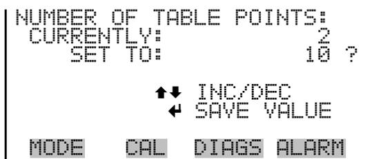
**Table Point** The Table Point menu allows the user to set up an individual table point.
