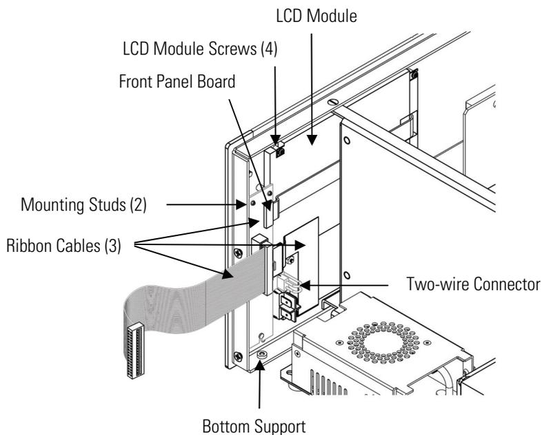
**Figure 7-14.** Replacing the Front Panel Board and the LCD Module
