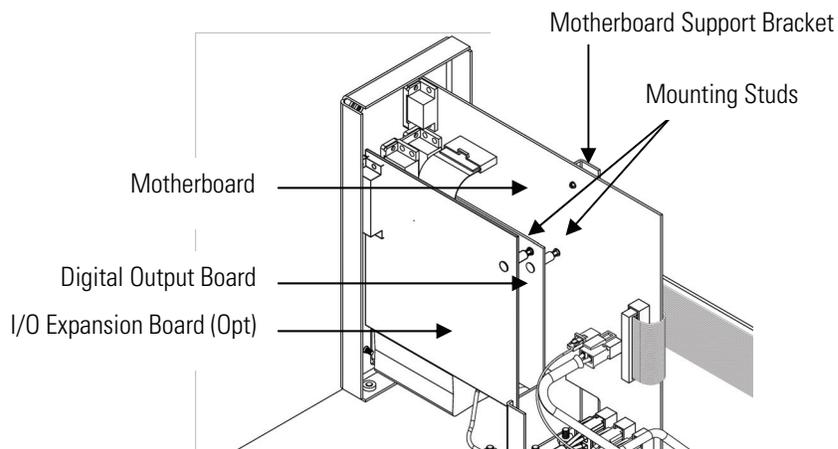
**Figure 7-11.** Replacing the I/O Expansion Board (Optional)
