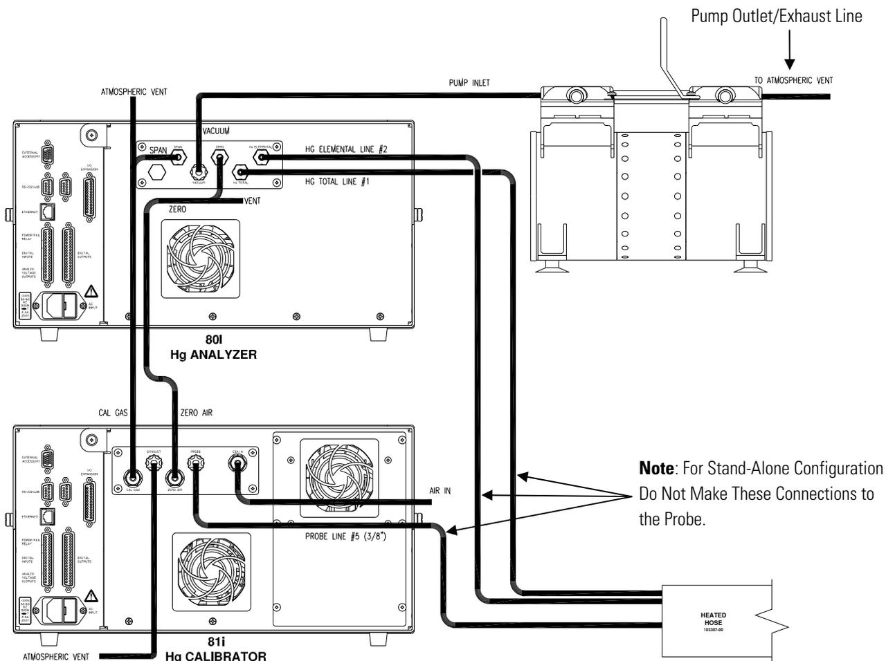
Figure 2-3. 80*i* and 81*i* Plumbing Connections
