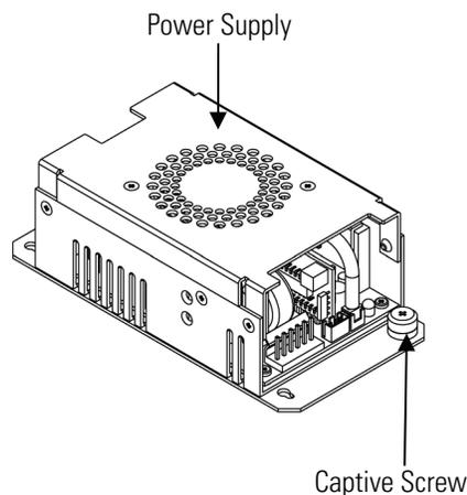
**Figure 7-7.** Replacing the DC Power Supply
